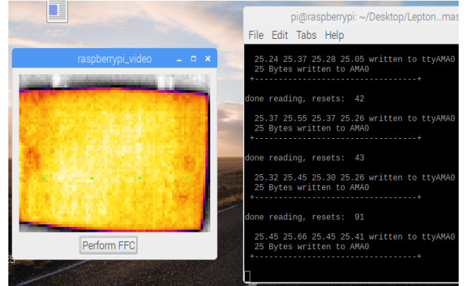
FIGURE 4: THERMAL IMAGE OF THE PELTIER MODULE WITH TEMPERATURE VALUES
