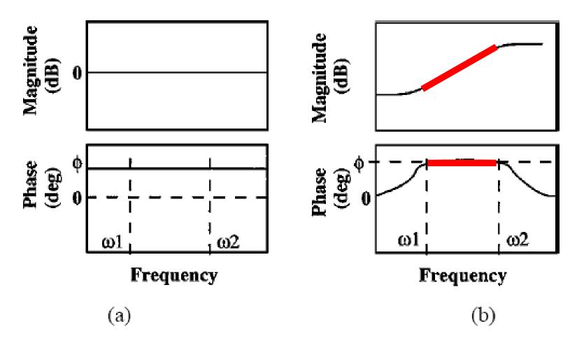
Fig. 10. Frequency response. (a) Ideal phaser. (b) Approximation.
