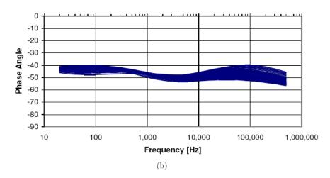
Fig. 1. Spectral response of the Fractor<sup>TM</sup> used in this demonstration project; (a) the impedance magnitude and (b) impedance phase. The multiple lines show the variation over 26 impedance measurement scans.
