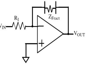
Fig. 2. Schematic for a fractional order integrator.  $Z_F$  represents the Fractor<sup>TM</sup> element. The schematic symbol for the Fractor<sup>TM</sup> was designed to give the impression of a generalized Warburg impedance; a mixture of resistive and capacitive characteristics.
