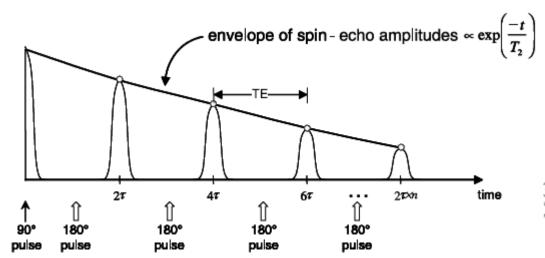
Carr–Purcell–Meiboom–Gill (CPMG) pulse sequence, as shown in Fig. 1, is widely used to measure spin-spin relaxation time T2
